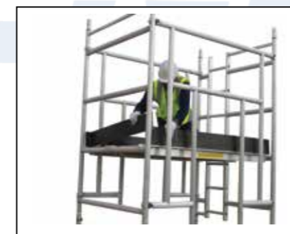
Step 14 Add toe boards to complete the structure. Slide the side board into the correct slot in the end boards, ensuring the object cannot fall through & the trapdoor can open fully.
