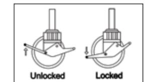
4)Wheel lock - Install castor / leg assembly to frame by pushing the leg into the frame tube. This Should be done with manual force only, no tools. Lock Castors before ascending any part of the tower.
